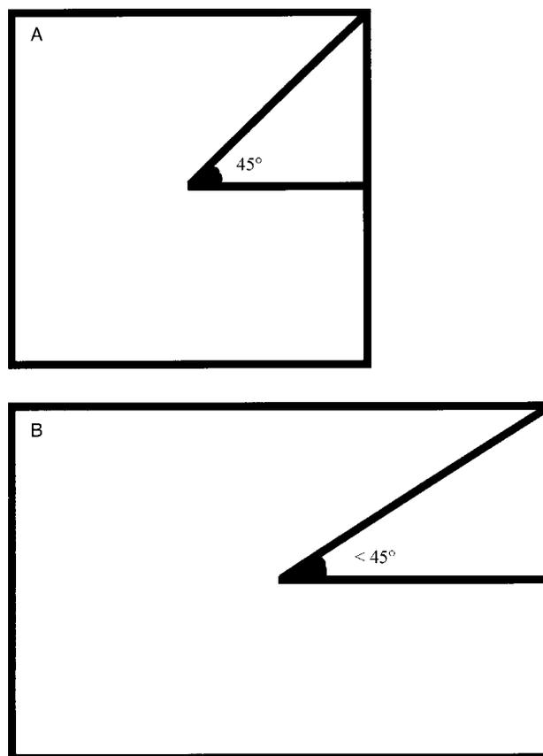
**Figure 7** Relation between the central angles formed by a square (object) and a rectangle (image formed by the panoramic radiograph)
